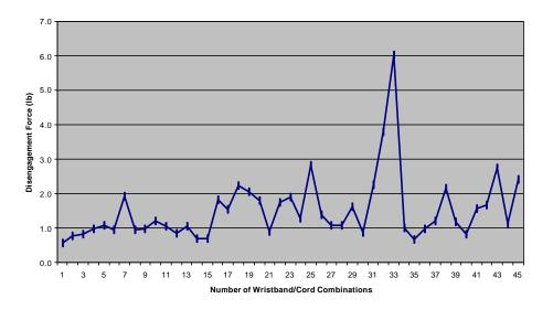
Figure 1. Breakaway Force Data for Wristbands with Formed Snaps
