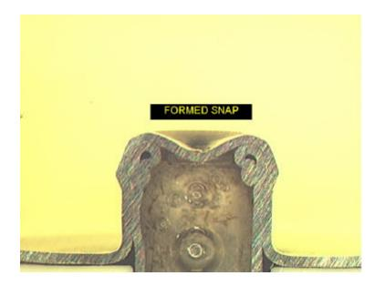
Figure 3. Cross Section of a Formed Snap
